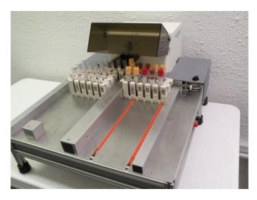
A detachable chute guides the caps into a disposal area beneath the instrument after decapping.
